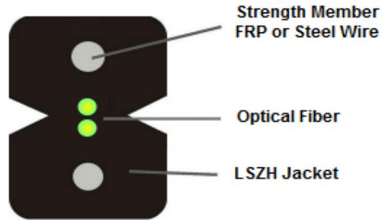
Remark: The weight of zinc coating of steel wire surface shall be no less than 20 g/m<sup>2</sup>. Strand shall have a left lay.
