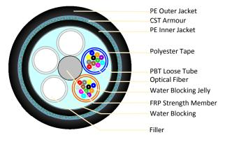
around to ensure consistent round. A inner Polyethylene (PE) sheath is applied to the overall bundle. It is further enhance by a layer of corrugated steel tape armour, longitudinally applied over the inner sheath. The cable is completed with a smooth Polyethylene (PE) sheath.
